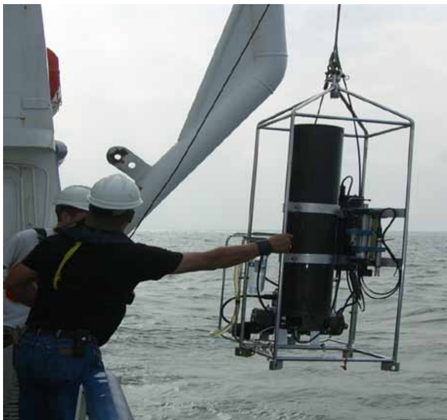
Deployment of portable membrane introduction mass spectrometer system for real-time, in-water chemical analysis of dissolved gases and volatile organic compounds.
