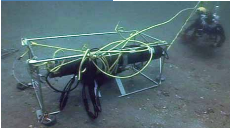
Recovery of the underwater mass spectrometer after a long-term deployment on the seafloor of the Atlantic Ocean.
