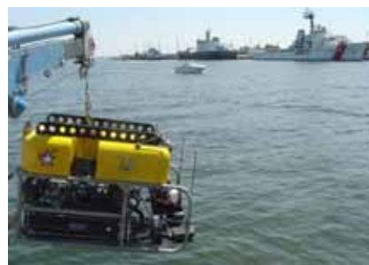
Remotely operated vehicle with sonar, camera and geo-positioning being readied for deployment.
